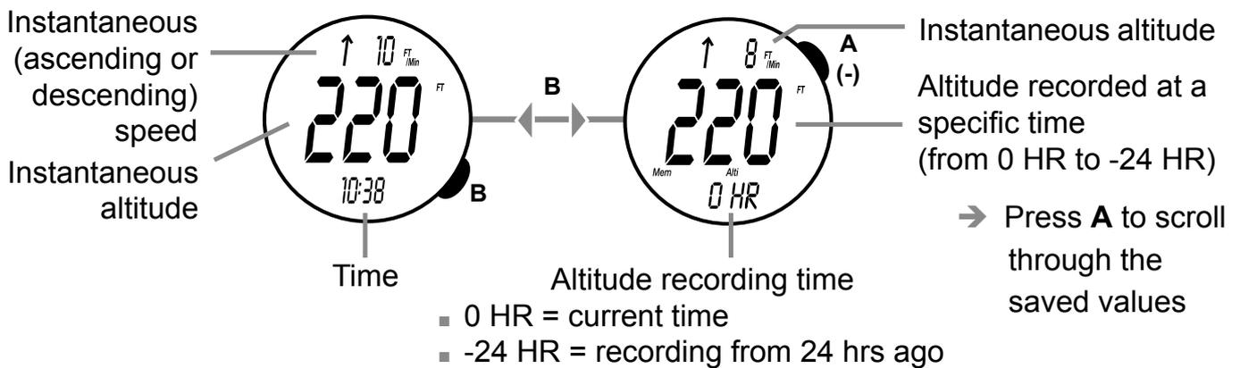
**Note:** The sensor is accurate to 1 metre (or 1 foot) and takes measurements between -700 m (-2296 ft) and +9,000 m (+29,520 ft). Changes in weather, even imperceptible ones, can affect the value displayed (1 mbar difference in pressure equals about 8 m in gradient). You will need to recalibrate the altimeter regularly.
