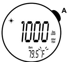
→ To change the temperature unit displayed (°C or °F), press and hold **A** until the display stops blinking.
